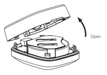
2, Push the old battery out and insert the new battery. Please note that the positive polarity should be upward and the negative polarity should be downward.
