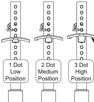
**!** The body hangers adjust the height of the body in 1.2mm steps. Note the dots on the underside.
