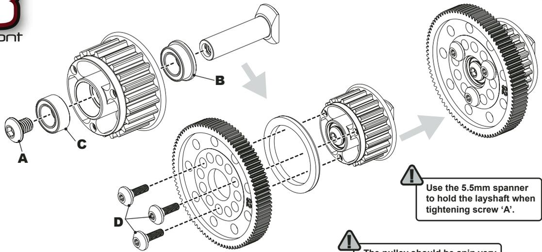
Use the 5.5mm spanner to hold the layshaft when tightening screw 'A'.
