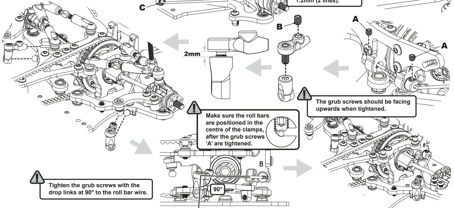
Tighten the grub screws with the drop links at 90° to the roll bar wire.
