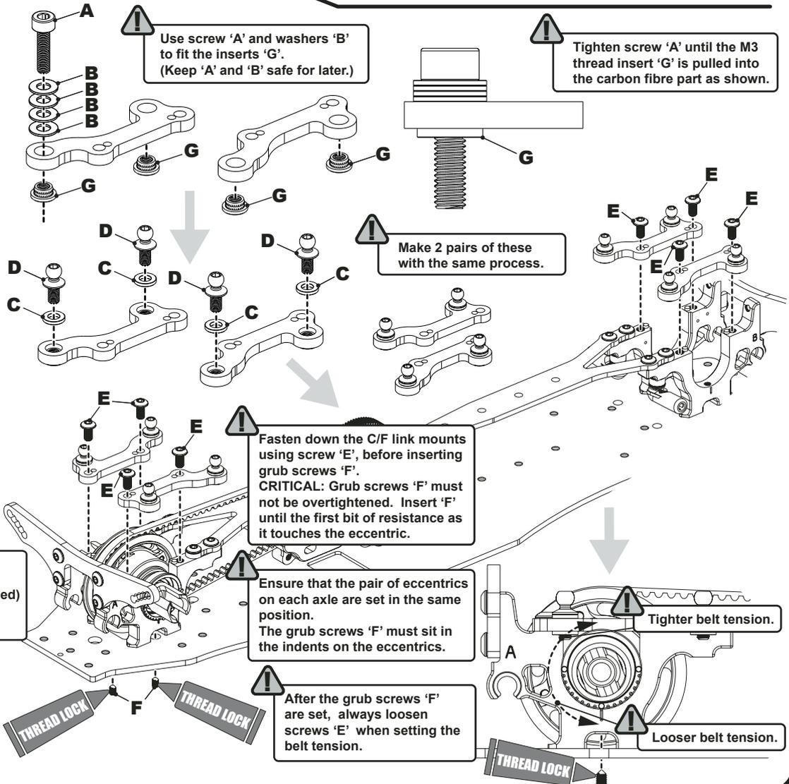
**!** Use screw 'A' and washers 'B' to fit the inserts 'G'. (Keep 'A' and 'B' safe for later.)
