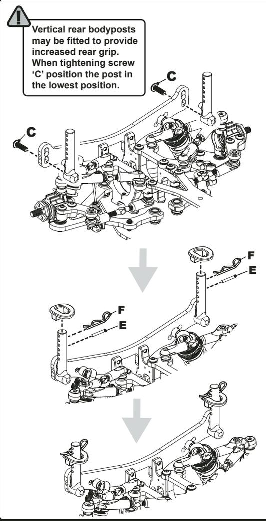
**!** Vertical rear bodyposts may be fitted to provide increased rear grip. When tightening screw 'C' position the post in the lowest position.
