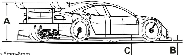
This allows to run the body lower to gain front downforce without excessive touching against the track surface. If you prefer not to use the body stop screws, set 'B' to between 8mm-9mm.
