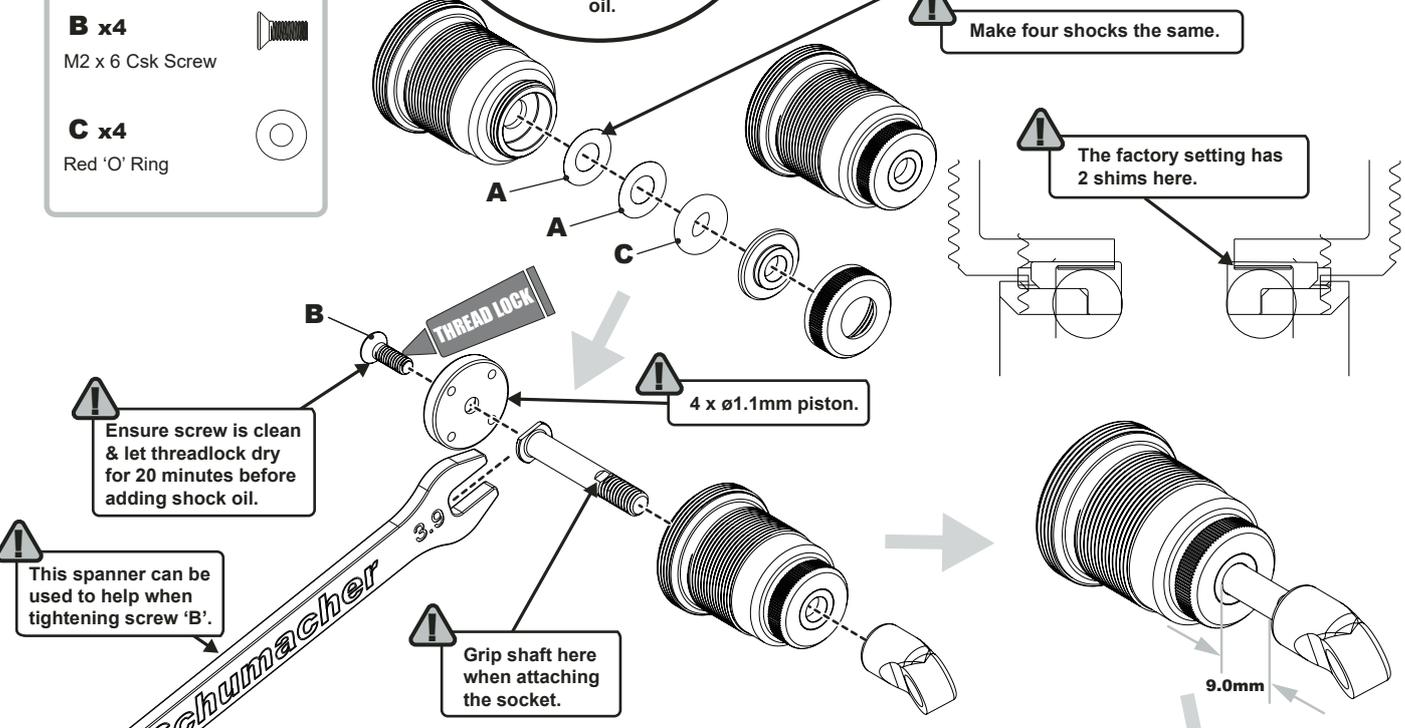
Drilling this hole through provides a 'vented' shock, and reduces the rebound.
