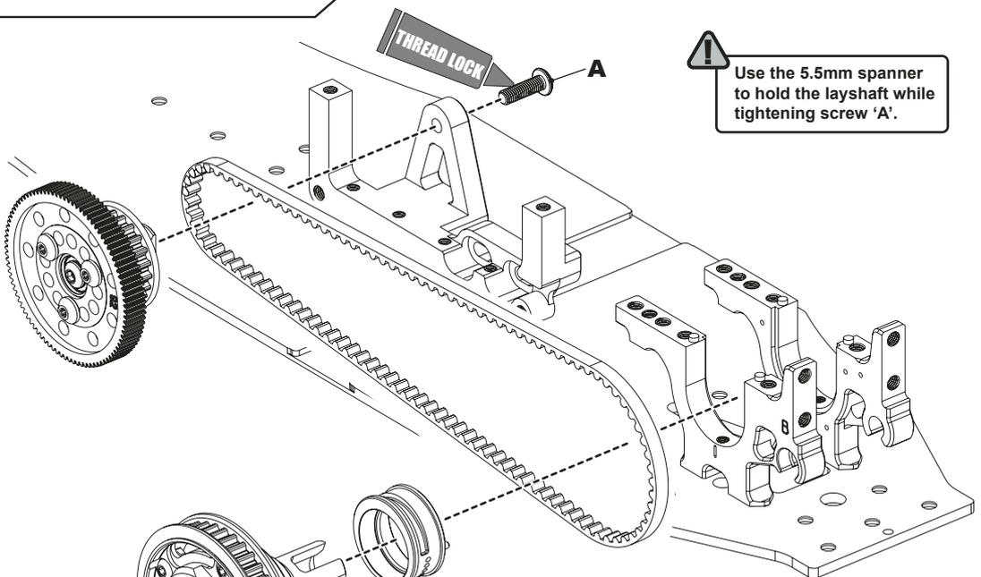
Use the 5.5mm spanner to hold the layshaft while tightening screw 'A'.
